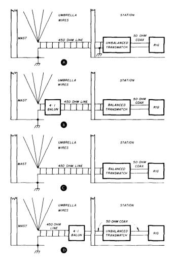
fig. 3. Transmatch and feedline configurations for the antenna. Sketch (A) shows the basic arrangement using an unbalanced transmatch. Note grounding. In (B) a balanced transmatch is used. A 4:1 balun is required. Sketch (C) shows an arrangement as in (B), but without the 4:1 balun. Transmatch is balanced (no ground). Sketch (D) shows how to use a short length of coax cable between the open-wire line and the station. The coax cable length should be as short as possible.
